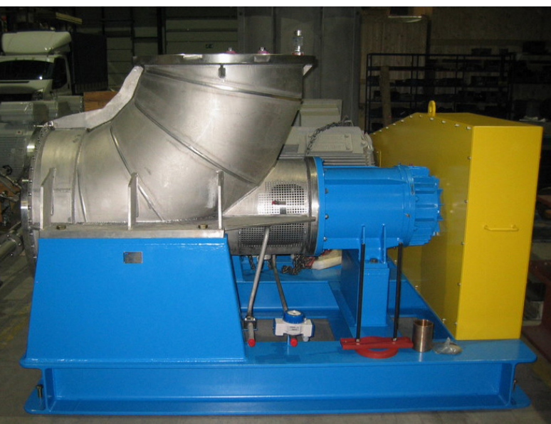
Evaporator circulation pump type CAHRM750K in workshop prior to packing (2010).
