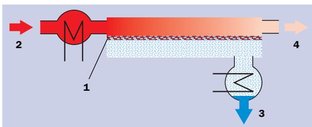
**1** The principle of pervaporation: By means of a semi-permeable membrane (1), water or methanol (3) is removed from the feed mixture (2) to provide a purified product (4).
