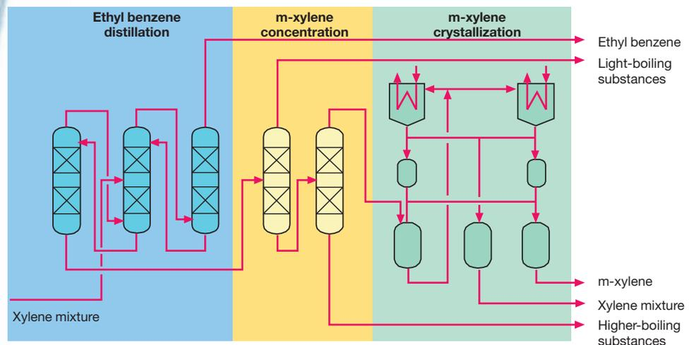
2<sup>■</sup> The process developed by Sulzer Chemtech for the purification of m-xylene is characterized by three steps: separation of ethyl benzene, concentration of m-xylene and the purification of m-xylene.
