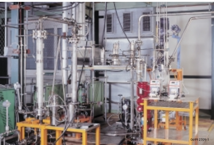
2 The process requirements of customers can be tested on a small scale in the Sulzer Chemtech pilot plant for polystyrene in Winterthur.
