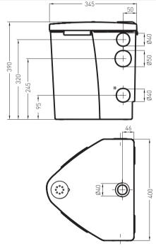
\* For Sanimax MF we recommend that the lower ports should not be used because the switch-on level is higher than the inflow level.
