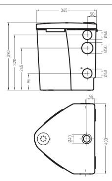
\* We recommend that the lower ports should not be used because the switch-on level is higher than the inflow level.
