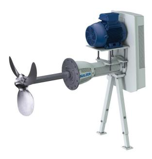
The new agitator is equipped with a new duplex stainless steel EX3 propeller for higher strength and wear properties. This ensures a longer lifetime than for agitators using austenitic stainless steel propellers. In addition, the performance of the agitator can be adapted with the adjustable propeller blades.
