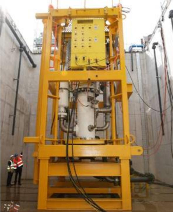
A complete pump/motor unit has been successfully tested at Sulzer Pumps' engineered test pool in Leeds, United Kingdom
