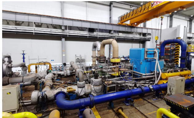
String testing of one of the feedwater pumps at Sulzer's manufacturing plant in Suzhou
