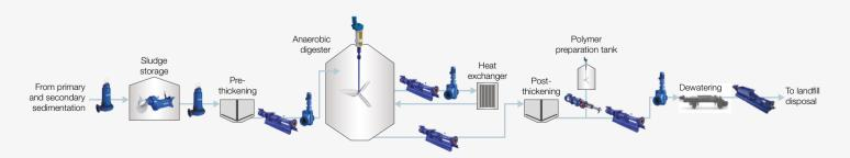
For AD systems, if the feedstock supply pump fails due to a blockage then the process starts to fail shortly afterwards. Without immediate attention, the bacteria responsible for breaking down the sludge and producing the methane will begin to decrease in number, reducing productivity.
