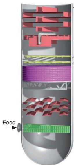
Upgrading a coker main fractionator to double the capacity, increase the liquid yield, and reduce the CCR of the HCGO from 0.4 to 0.3 %wt
