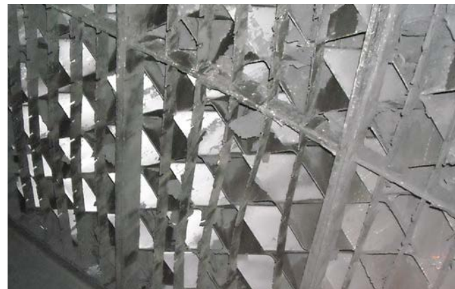
Mellagrid high-performance structured grid after 3 years operation, only small amount of coke at the bottom of the bed, washed in place and reused
