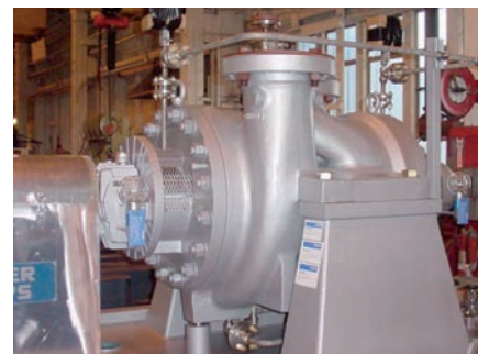
BBS: Single Stage Between Bearing, typically used at high temperature, high flow and high head, that is residue and bottom Pump Around of main fractionators
