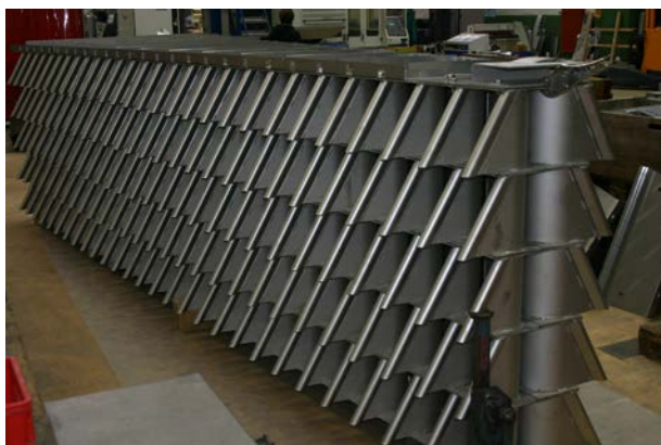
Shell SchoepentoeterPlus: the radial advanced feed inlet vane device for the flash zone
