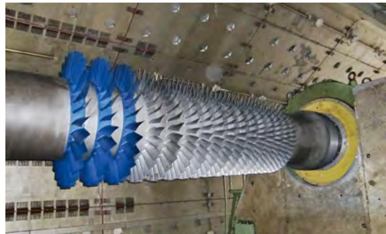
Fig. 2 Increasing the lifetime of rotor blades — metallic-ceramic coating in blue.
