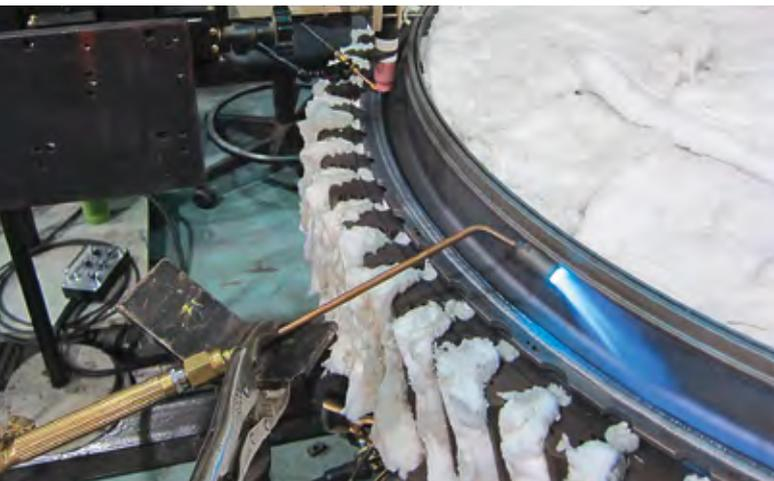
Fig. 1 Sulzer developed a proprietary welding procedure — gas-tungsten arc welding—for gas turbine repair.
