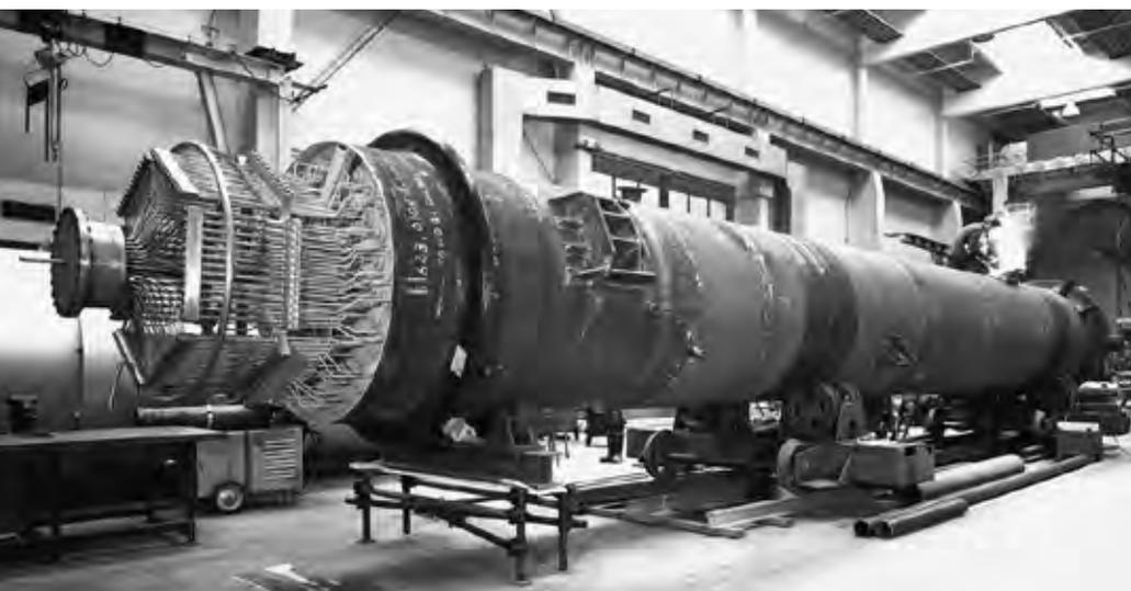
Fig. 1 Rectification apparatus (Kuhn column) from Sulzer.
