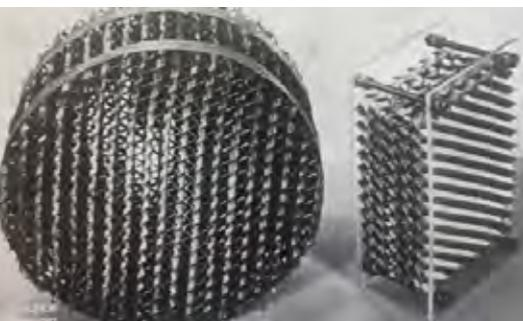
Fig. 4 The first generation of Sulzer gauze packing BX.
