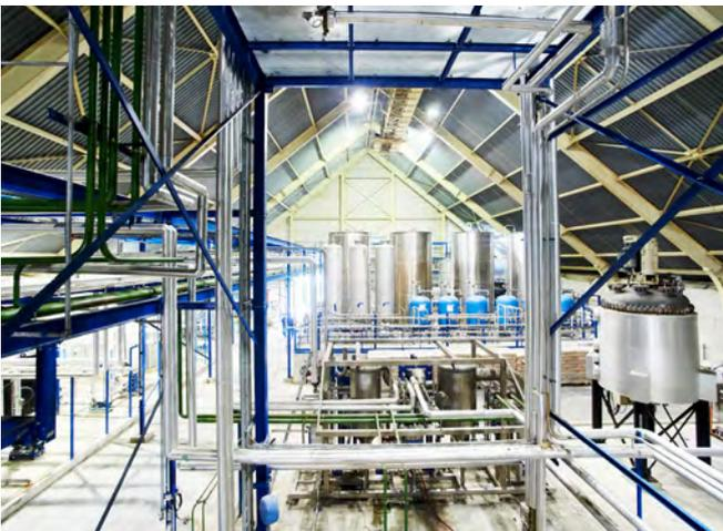
Fig. 2 Lactic acid process installation from Futerro (Source: Futerro).
