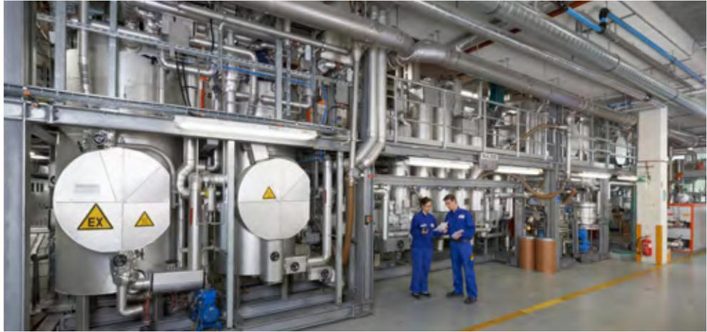
Fig. 4 Skid mounted unit for PLA production.
