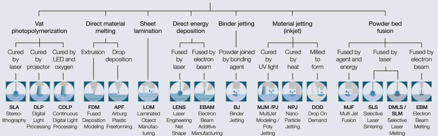
Fig. 1 Overview of the most important additive manufacturing technologies in the industrial sector.
