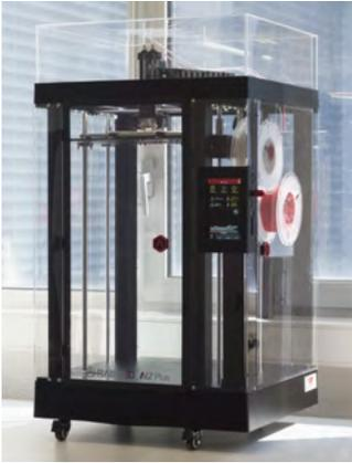
Fig. 3 Fused Deposition Molding (FDM) printer working with red-colored PLA.
