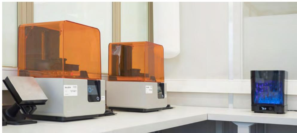
Fig. 2 Two stereolithography printers (left) and UV curing system (right).
