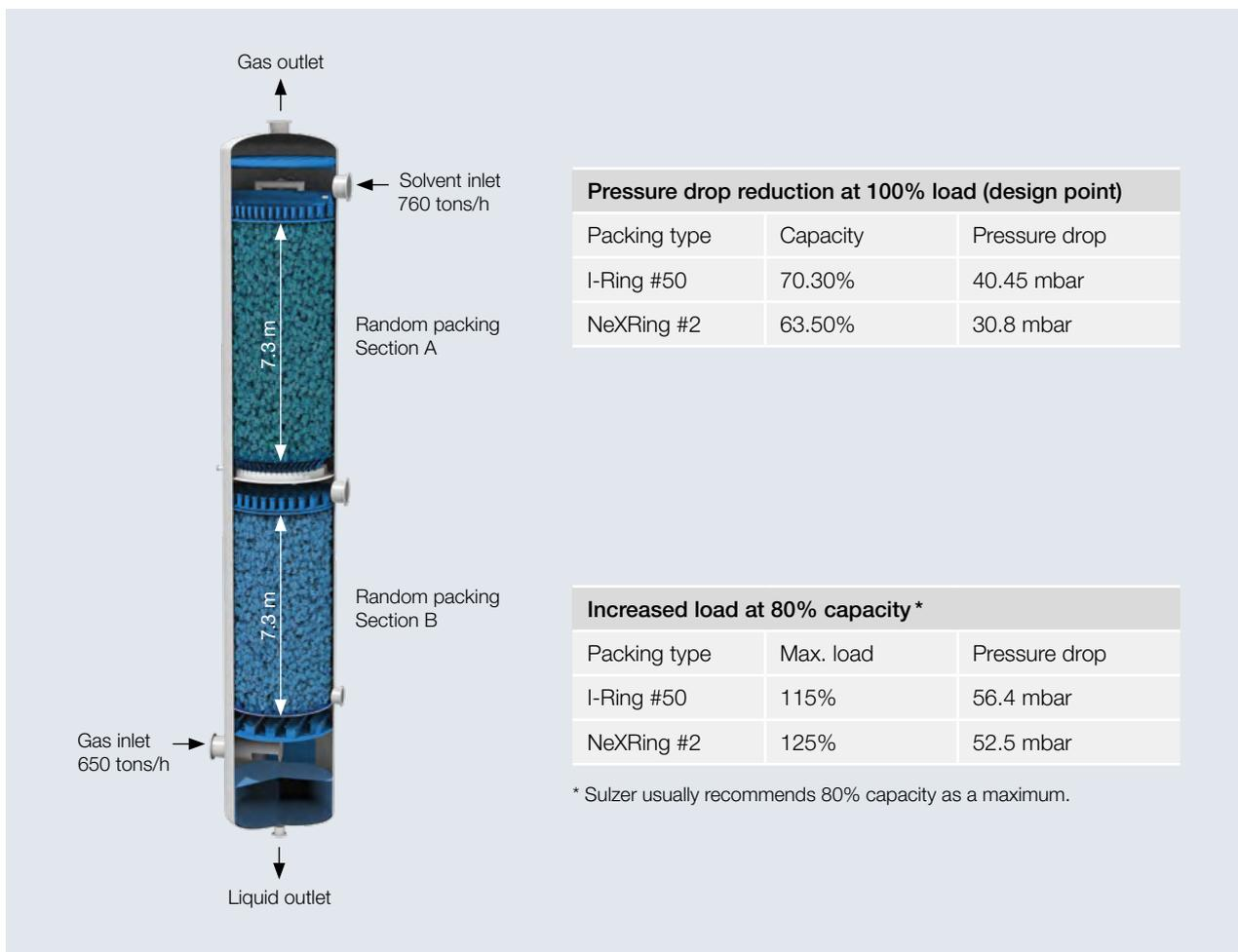
Fig. 2 Carbon dioxide absorption column – comparison of values with I-Ring and NeXRing.
