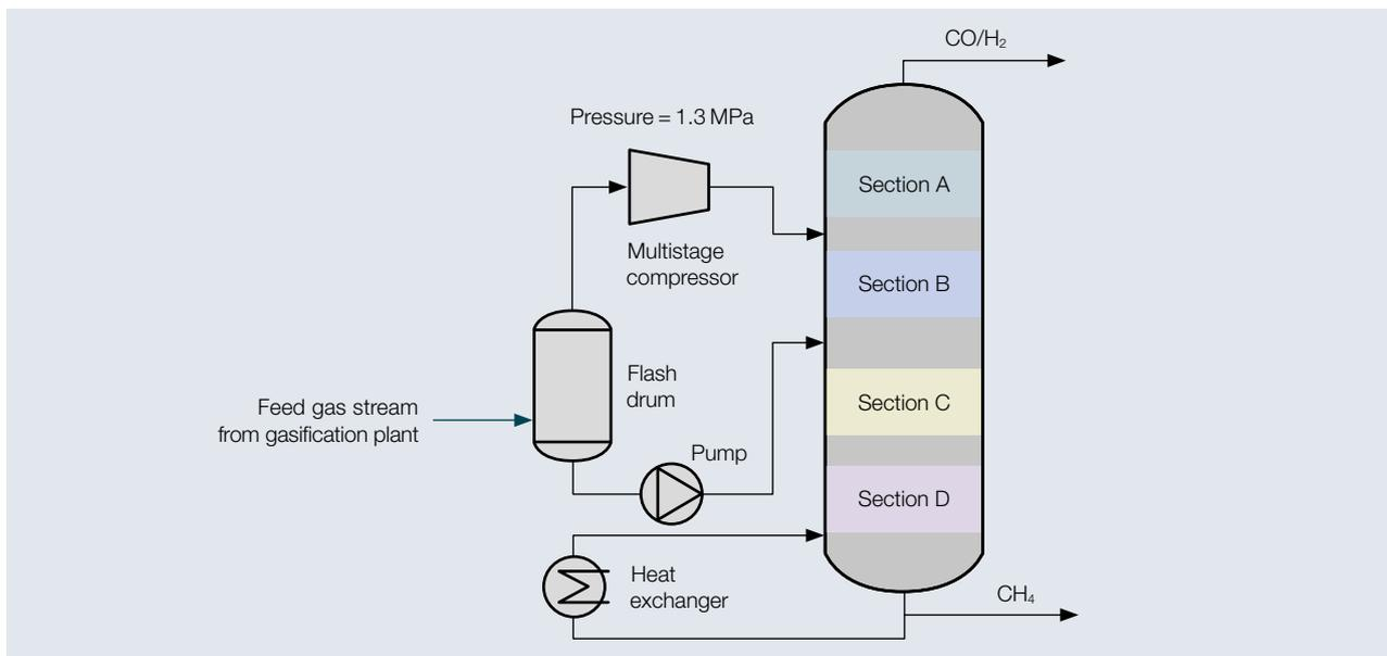
Fig. 3 Process workflow of a methane separation installation.
