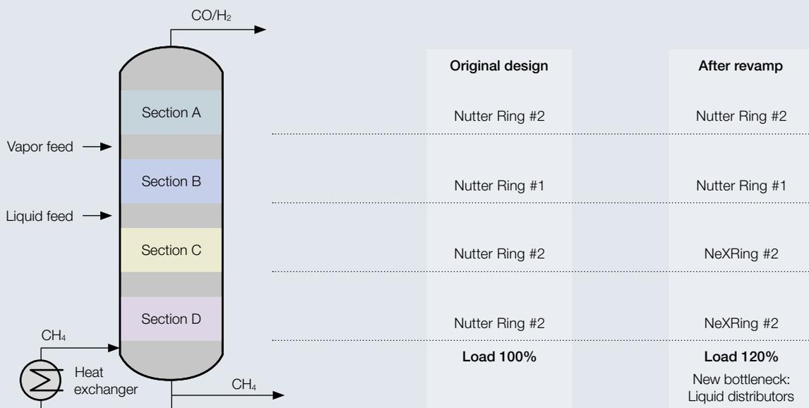
Fig. 4 NeXRing improves the capacity for methane separation.
