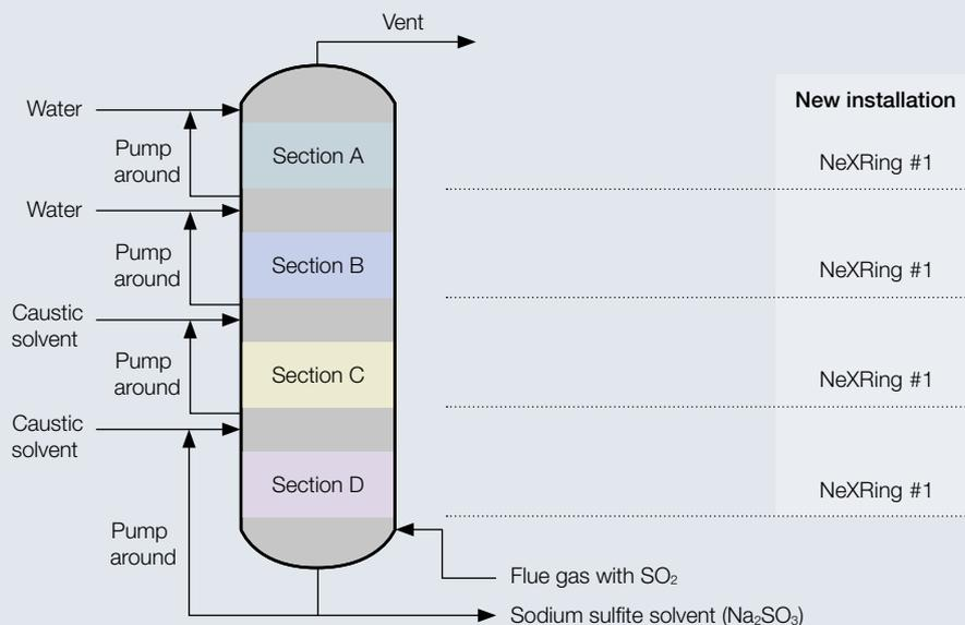
Fig. 6 NeXRing in a flue gas treatment column to reduce SO<sub>2</sub>.
