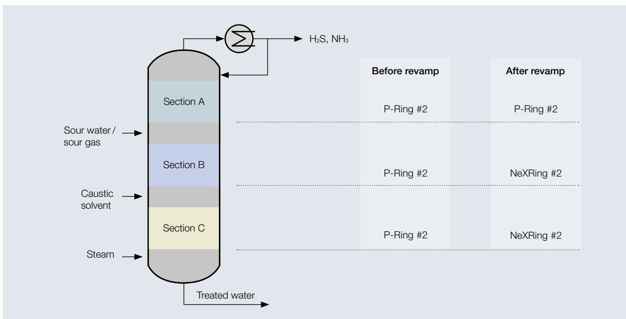
Fig. 5 Less fouling thanks to NeXRing in wastewater stripping tower.
