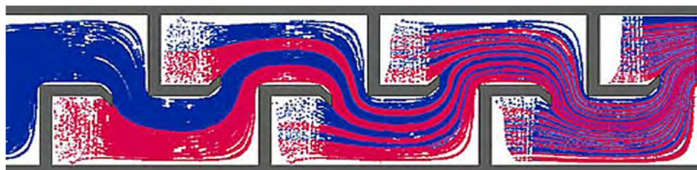
Fig. 4 Schematics of layer generation and mixing within laminar static mixers.
