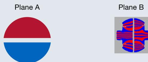
Fig. 8 Prediction of mixing pattern of a static mixer with the Sulzer in-house tool.
