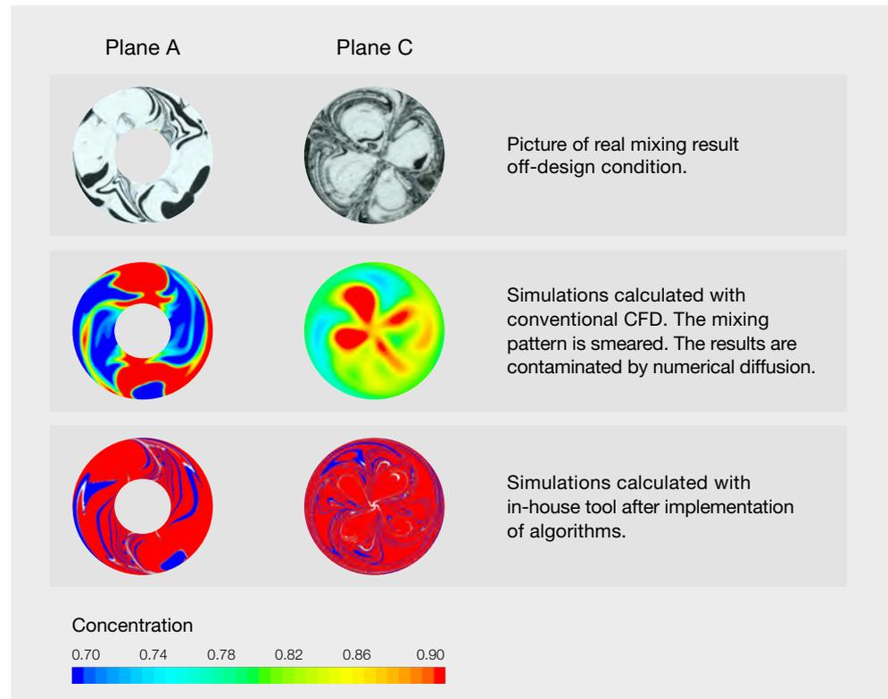
Fig. 10 Comparison of real mixing results with conventional CFD and in-house tool for dynamic mixers.
