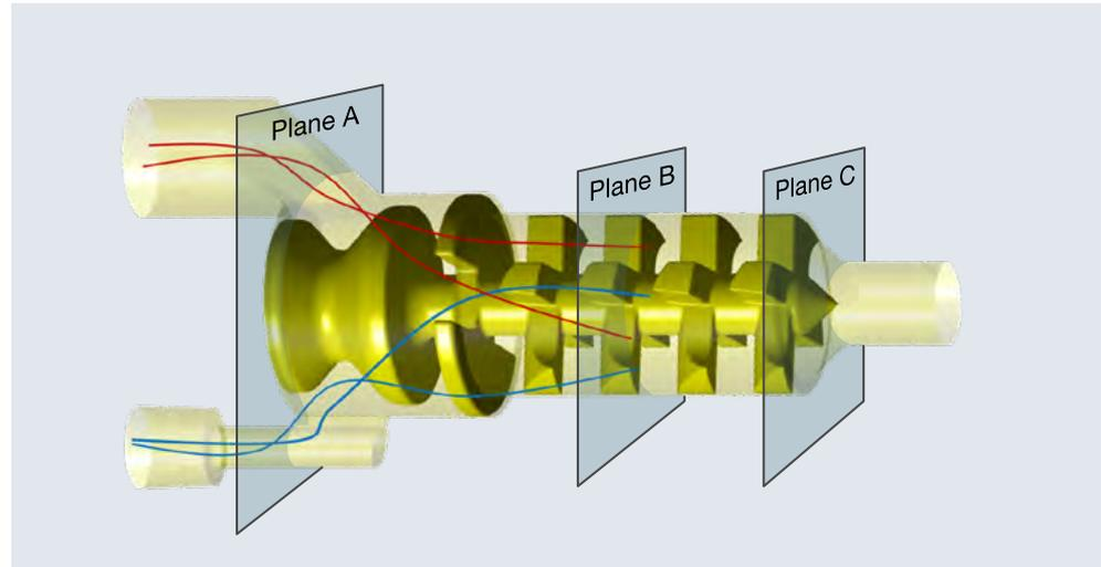
Fig. 9 Dynamic mixer – blue and red lines symbolize the particle tracking.
