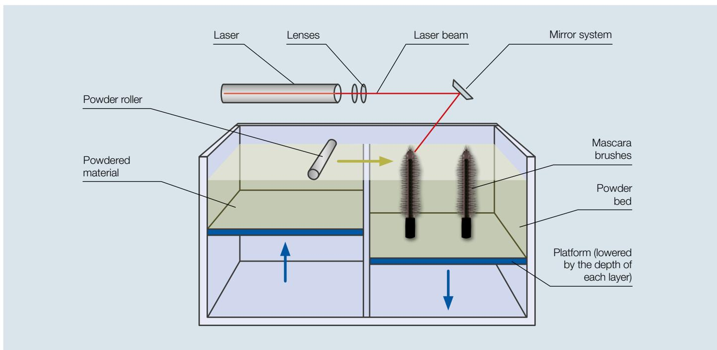
2 Functional principle of the selective laser sintering process, also called SLS.
