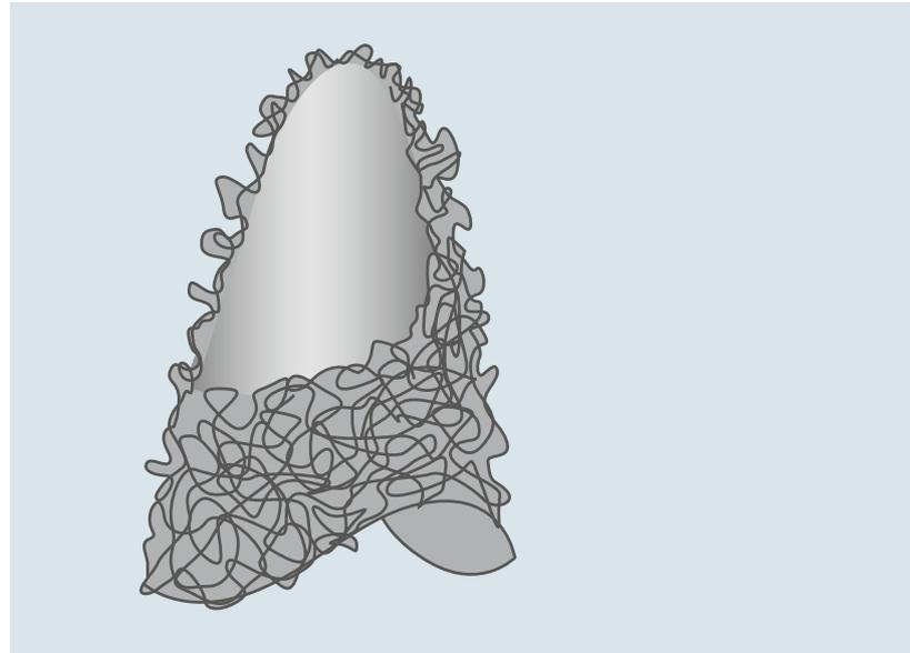
3 Schematic view of a prototype of a mascara brush bristle tip using laser sintering (SLS).
