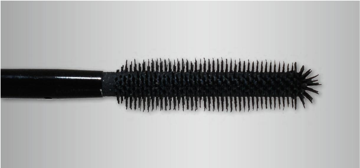
1 Prototype of a mascara brush made using the 3D-printing process.
