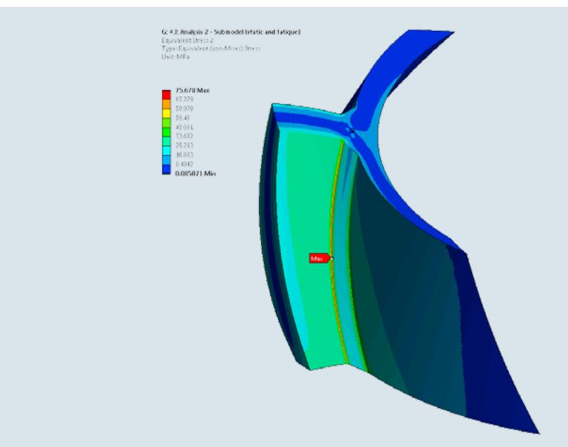
5 Finite element analysis of weld seam to check the feasibility.
