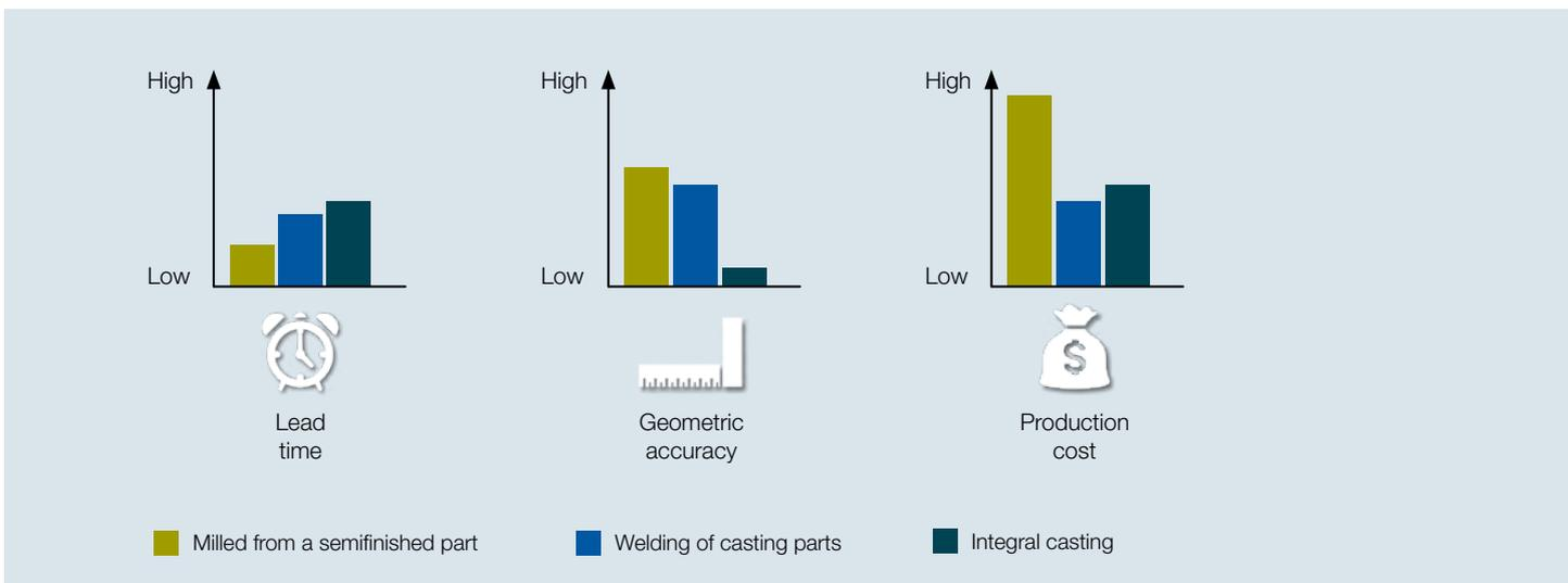
4 Comparison of three manufacturing methods for large vertical impellers.
