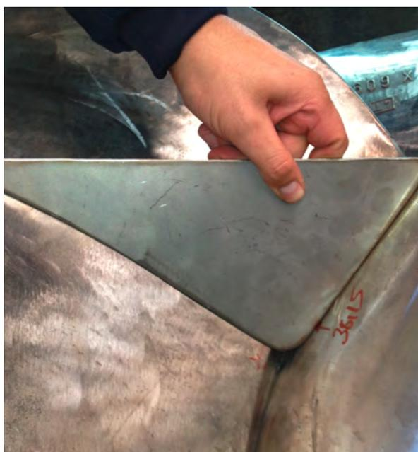
7 Positioning template for the blades used during the welding process.
