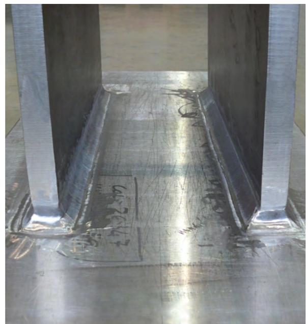
6 Welding model to test the weld quality and check the geometry.
