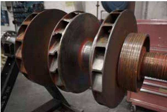
2 Severe damage to the second-stage impeller and labyrinth seals.
