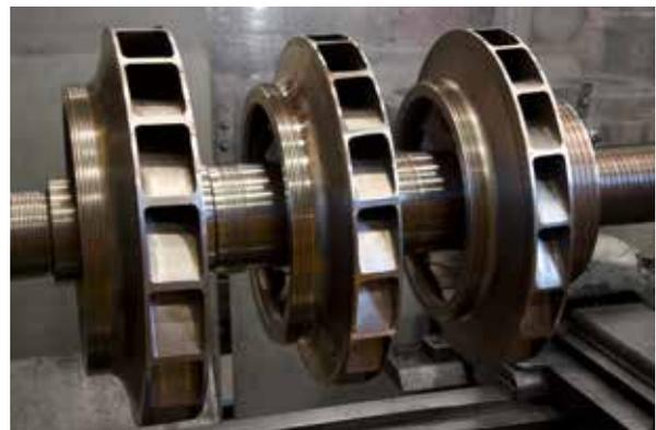
3 The new impeller before being precision balanced.
