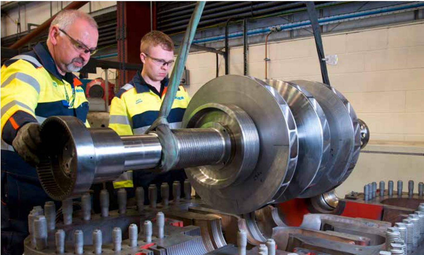
1 Final inspection of the repaired compressor in Leeds.
