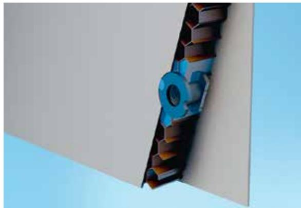
3 Illustration of bonding an insert into a composite sandwich panel. (Source: DELO)
