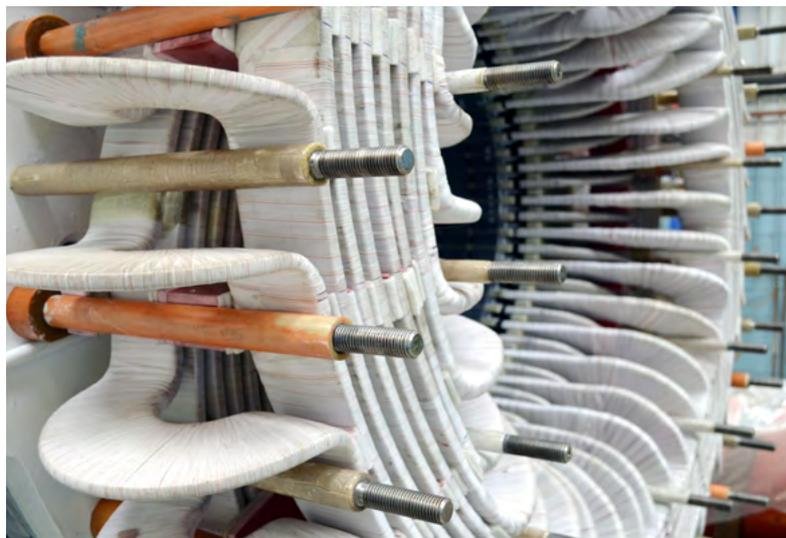
3 Precise fitting of 72 hairpin coils inside the generator.
