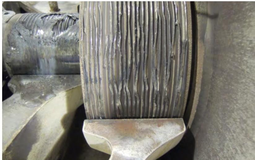
3 Shaft and balancing piston labyrinths.
