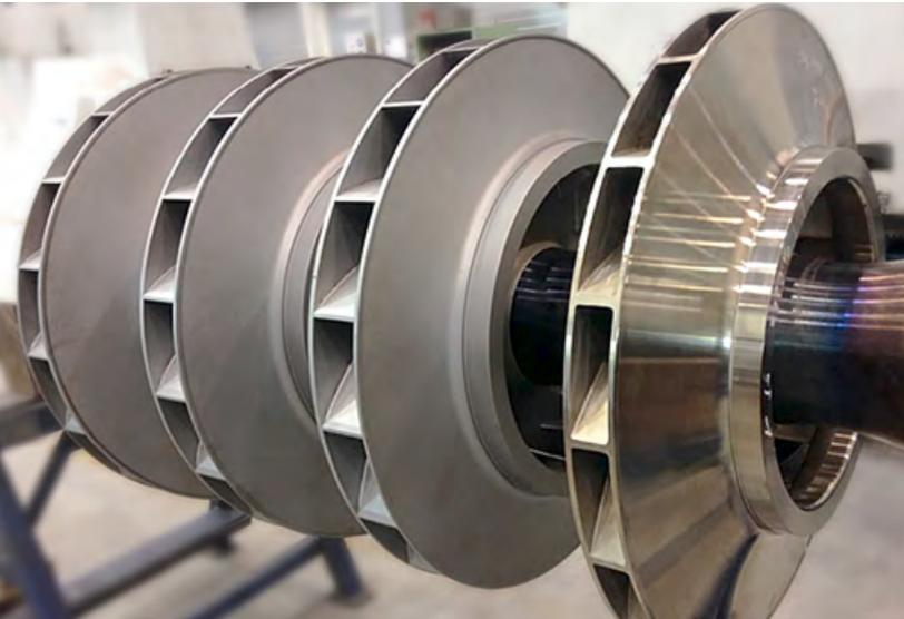
5 Repaired in Rotterdam – the rotor with one new impeller.
