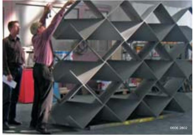
**3** The Sulzer Chemtech SMV gas mixer creates low pressure drop and delivers an excellent mixing performance.
