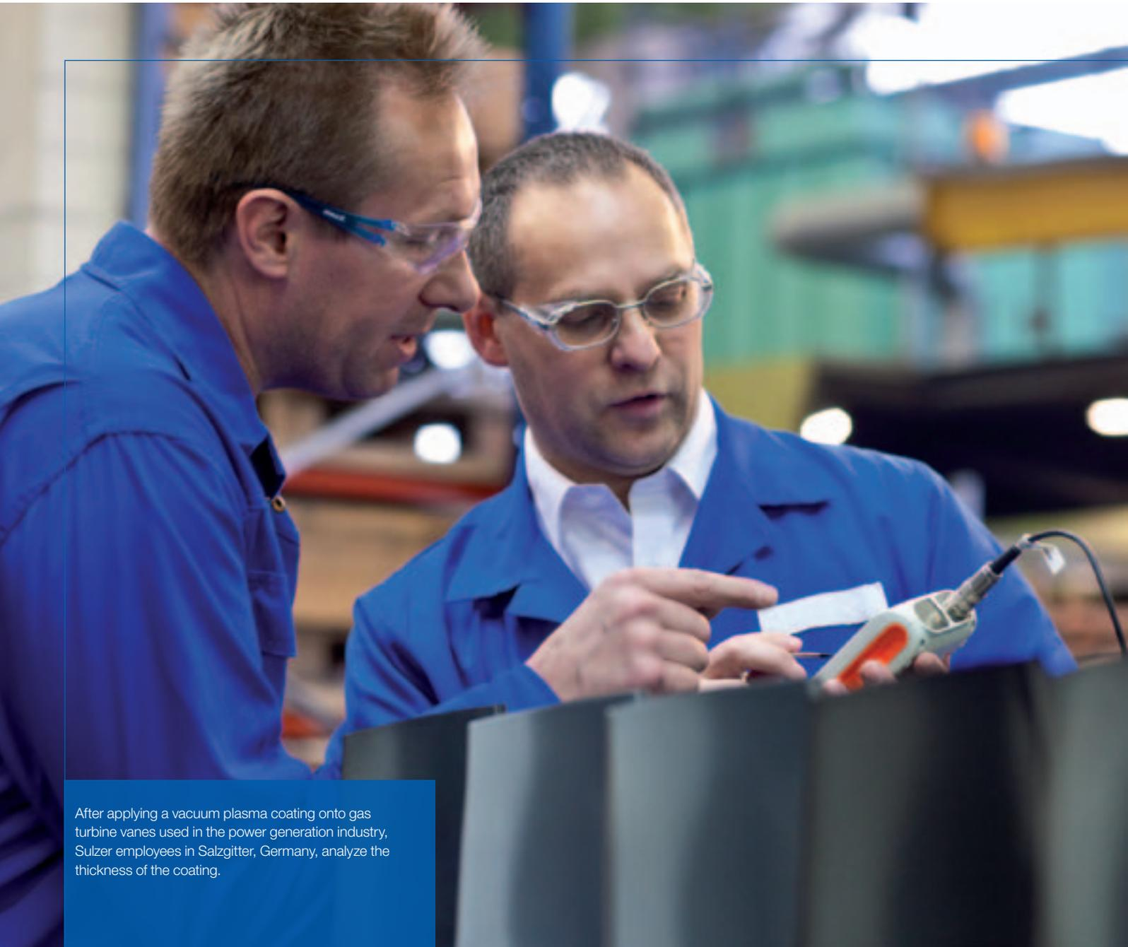
After applying a vacuum plasma coating onto gas turbine vanes used in the power generation industry, Sulzer employees in Salzgitter, Germany, analyze the thickness of the coating.
