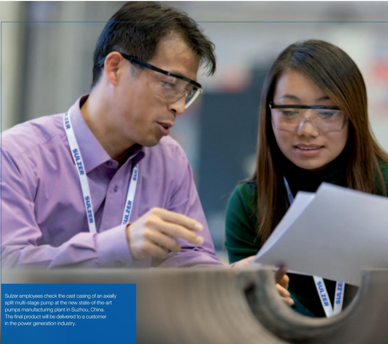
Sulzer employees check the cast casing of an axially split multi-stage pump at the new state-of-the-art pumps manufacturing plant in Suzhou, China. The final product will be delivered to a customer in the power generation industry.
