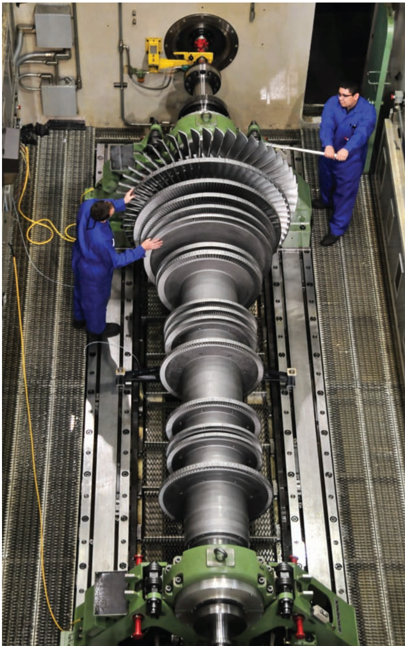
4 High-speed steam turbine, typical of the type requiring high-speed balancing.
