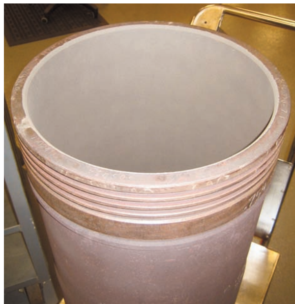
7 Large bore liner (317.5 mm diameter) after coating.
