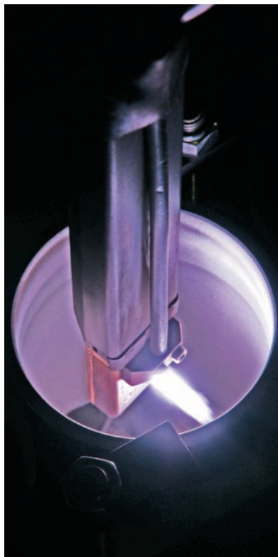
5 Coating of a cylinder bore of a diesel engine with the F210 APS gun.
