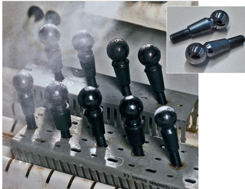
3 Sulzer Metaplas treats ball studs for all well-known European vehicle manufacturers.
