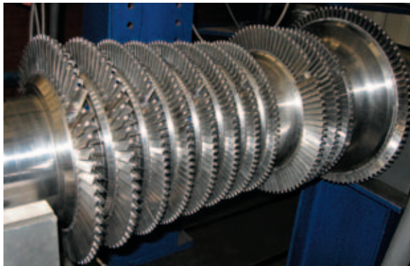
The blades being installed in the new rotor.
