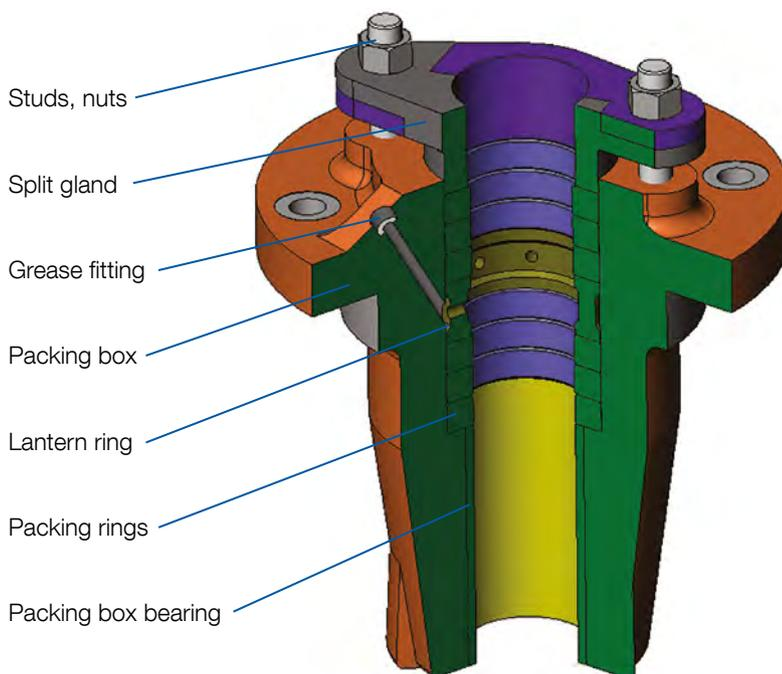
NOTE: When repacking a packing box, be sure to clean out the old packing, including the packing below the lantern ring. Packing box is provided with a provision for a grease fitting but greasing is at the discretion of the operator. Standard packing provided by Sulzer only requires product lubrication.
