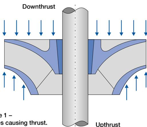
Figure 1 – Forces causing thrust.
