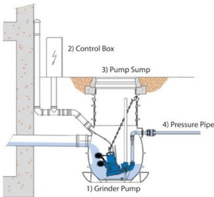
**Grinder pumps typically range from 1.3 to 2.6 kW, depending on the flow rate required**
