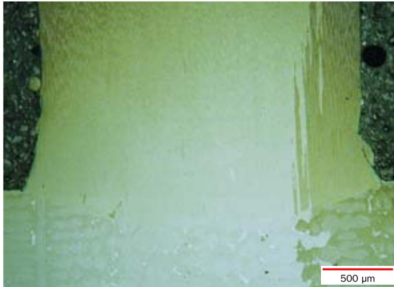
**2** This micrograph shows the weldability of high gamma prime DS material (a nickel base casting): The DS structure of the GTD-111 alloy (bottom) is continued in the weld. The filler metal is Inconel 738 LC.
