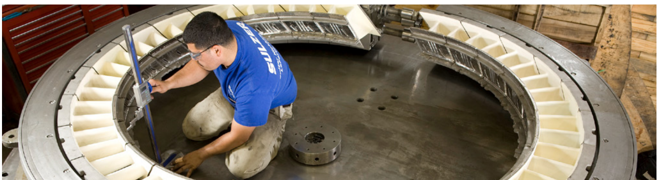
501F vane final assembly
