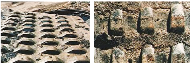
2-pass VG AF trays with V-Grid, sloped outlet weir and push valves.
