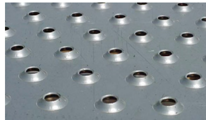
Extruded holes from liquid-liquid extraction holes
