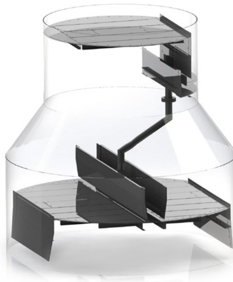
Transition from a 1-pass tray to a 2-pass tray over a conical section.
