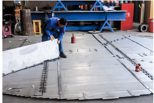
Shell CS Grid™ trays equipped with round bars
