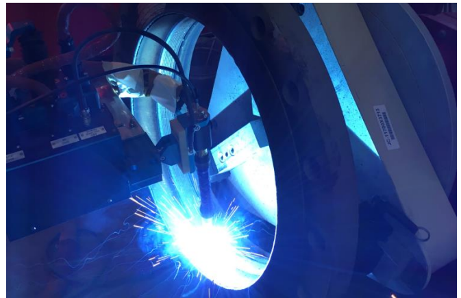
Picture 2: New build nozzle with automated weld overlay
